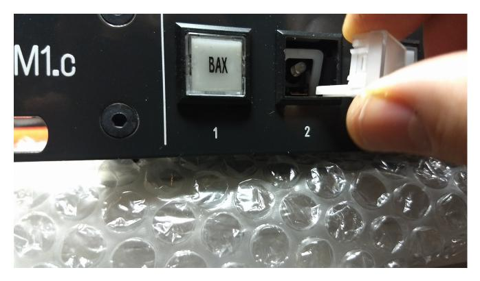
Gently push the knife point in so that the right side of the cover comes a bit loose. You can wiggle it a bit on the left side at the same time and the complete cover assembly comes loose and you can slowly pull it out.
