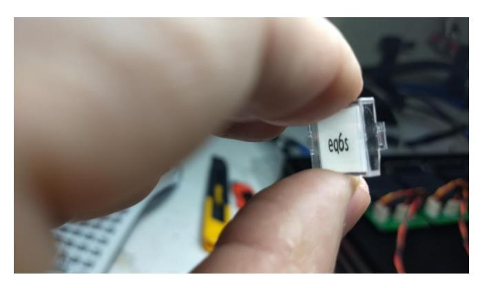
Now gently put the transparent lens-cover back on the white actuator base with the actuator pin facing to the bottom. Make sure that the locking pins on the side are put in the right place and not bend. You could gently push in the locking mechanism pins a bit so that they are 'clicking' into place but be careful.
