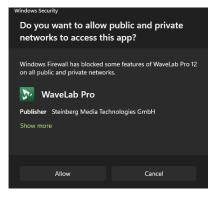
It's important that understand that the Insert Computer and your DAW need to connected to the same network, so they can see each other. By default, the IC2.1 is set to DHCP so it gets an IP address automatically and the plugin searches for a unit in the same network. This will work fine, but you might want to make a DHCP reservation or use a fixed IP address. This will speed the first time connection slightly up.
