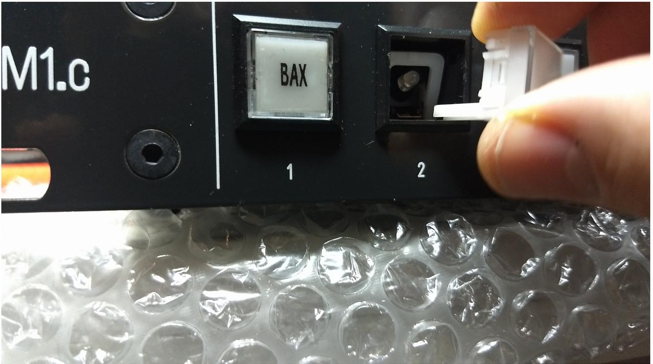
Gently push the knife point in so that the right side of the cover comes a bit loose. You can wiggle it a bit on the left side at the same time and the complete cover assembly comes loose and you can slowly pull it out.
