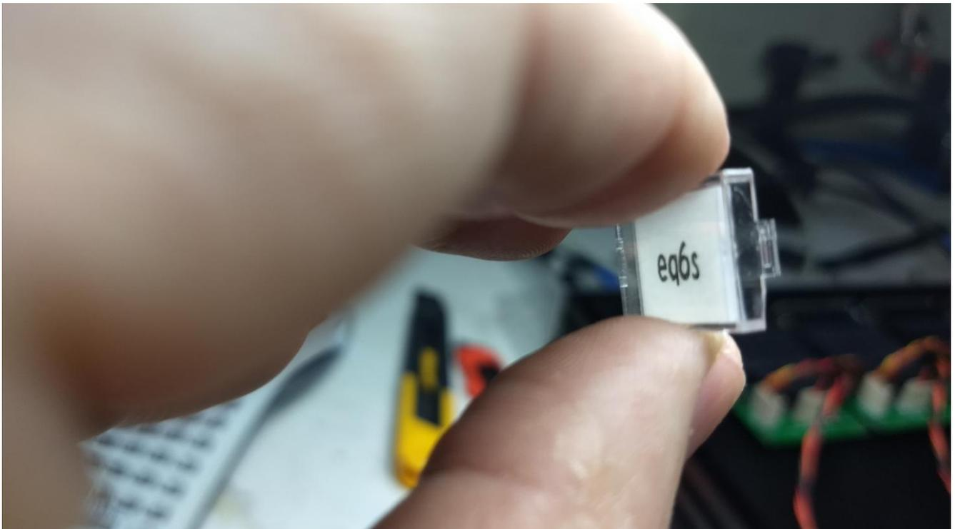
Now gently put the transparent lens-cover back on the white actuator base with the actuator pin facing to the bottom. Make sure that the locking pins on the side are put in the right place and not bend. *You could gently push in the locking mechanism pins a bit so that they are 'clicking' into place but be careful.*
