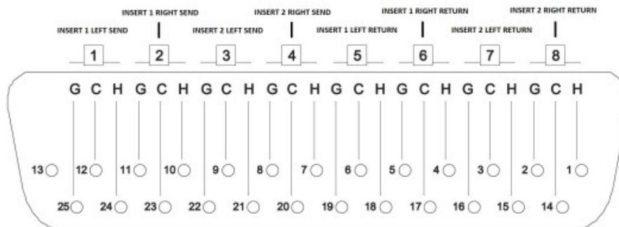
\* Note: Be careful with DB25 tascam standard/premade cables. The digital AES/EBU cables have their inputs and outputs swapped compared to the analog version.
