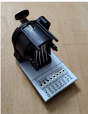
Optional PCB with Neutrik RJ45 connector In schematic J3 is the connector on PCB
